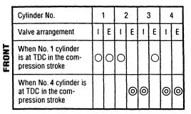
**3.** After adjusting the valves with piston No. 1 at TDC, rotate the crankshaft 360° again aligning the TDC mark and the pulley mark. This brings piston No. 6 or No. 4 to TDC, then adjust the remaining valves.
