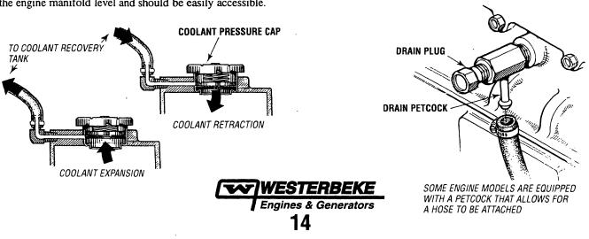
**NOTE:** Periodically check the condition of the manifold pressure cap. Ensure that the upper and lower rubber seals are in good condition and check that the vacuum valve opens and closes tightly. Carry a spare cap.
