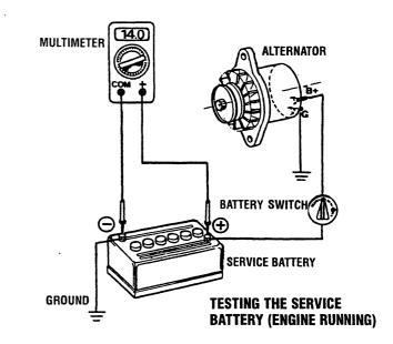
**CAUTION:** To avoid damaging the alternator diodes, do not use a high voltage tester (i.e. a megger) when performing tests on the alternator charging circuit.
