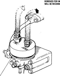
APPLY A THIŃ COAT OF CLEAN OIL TO THE O-RING WHEN INSTALLING THIS KIT. THREAD THE KIT ON, THEN HAND TIGHTEN AN ADDITIONAL 3/4 TURN AFTER THE O-RING CONTACTS THE BASE. To install, simply remove the engine oil filter and thread on WESTERBEKE's remote oil filter kit as shown. Always install this kit with the oil filter facing down as illustrated.
