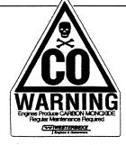
A WARNING DECAL is provided by WESTERBEKE and should be fixed to a bulkhead near your engine or generator. WESTERBEKE also recommends installing CARBON MONOXIDE DETECTORS in the living/sleeping quarters of your vessel. They are inexpensive and easily obtainable at your local marine store.
