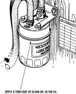
APPLY A THIN COAT OF CLEAN OIL TO THE FIL-TER GASKET WHEN INSTALLING. AFTER THE FILTER CONTACTS THE BASE, TIGHTEN IT AN ADDITIONAL 3/4 TURN.
