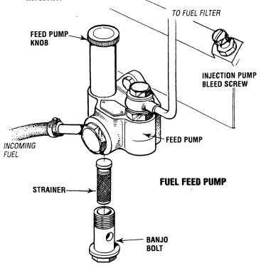
After changing the fuel filter and cleaning the fuel feed pump strainer, WESTERBEKE recommends the following procedure for ensuring there is no air trapped in the fuel system.
